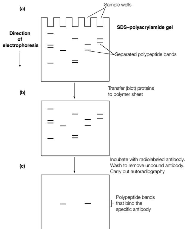
*Fig. 2. Immunoblotting using a radiolabeled antibody (a) SDS polyacrylamide gel electrophoresis, yielding polypeptides separated into discrete bands; (b) nitrocellulose or nylon membrane onto which the protein bands have been blotted (i.e. a Western blot); (c) autoradiograph after incubating the Western blot with radiolabeled antibody, washing away unbound antibody and placing the membrane against X-ray film.*
