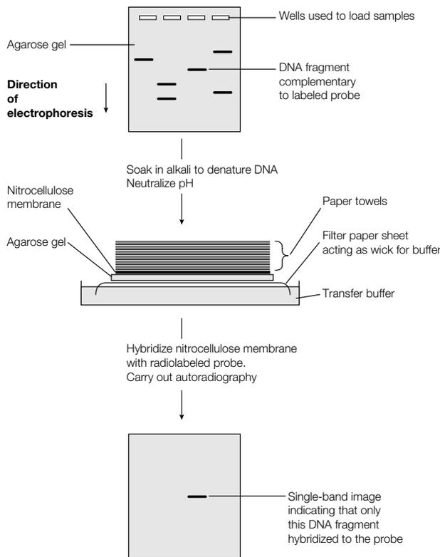
*Fig. 1. Southern blotting. The procedure shown is the original method of Southern using capillary action to blot the DNA bands from the gel to the nitrocellulose membrane. Electrolytic transfer is now often used instead.*
