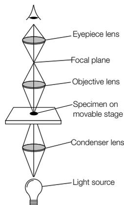
*Fig. 1. Optical pathway of a compound microscope.*
