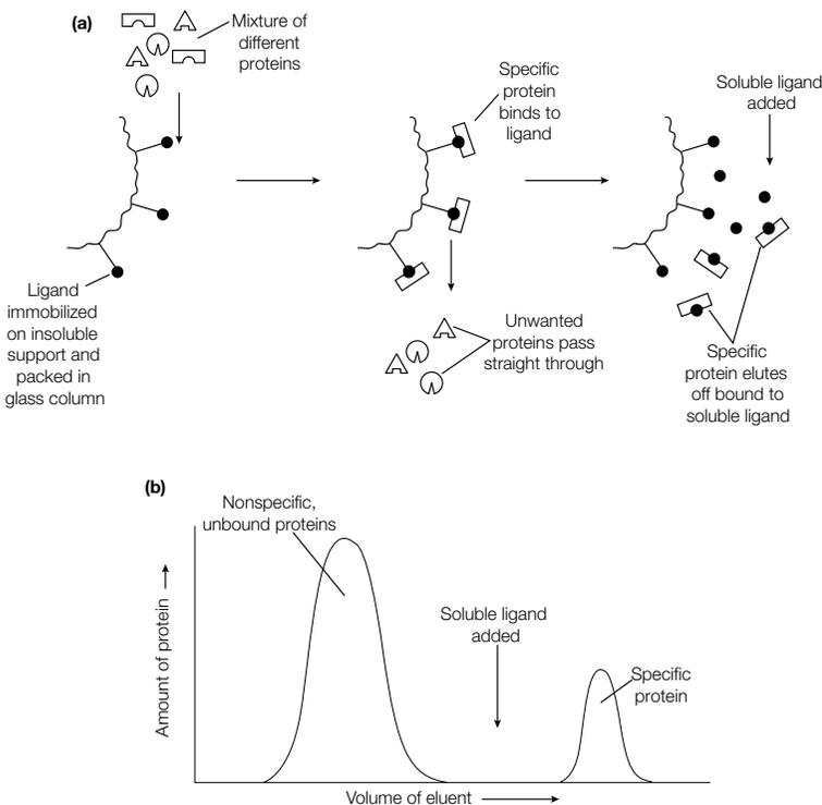
Fig. 4. Affinity chromatography. (a) Schematic diagram of affinity chromatography; (b) elution diagram indicating that nonspecific proteins that do not bind to the immobilized ligand pass straight through the column, while the specific protein binds to the immobilized ligand and is eluted from the column only on addition of soluble ligand.
